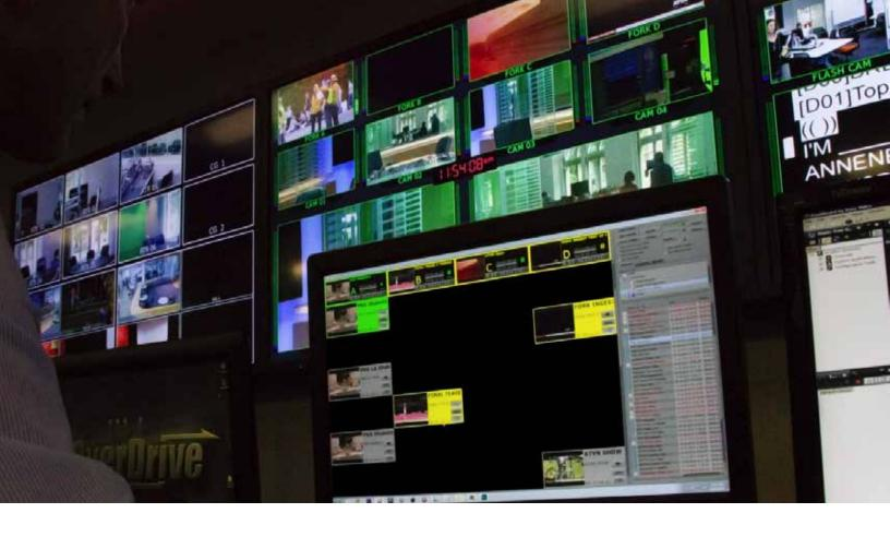
The Media Center's ingest environment pulls content from satellite, local studio, and VTR sources through an HD Miranda router onto video servers running FORK Ingest HD. From there it's transcoded into a universally recognized file format (XDCAM) and then distributed across a GigE local area network to the central storage and tape archive.
